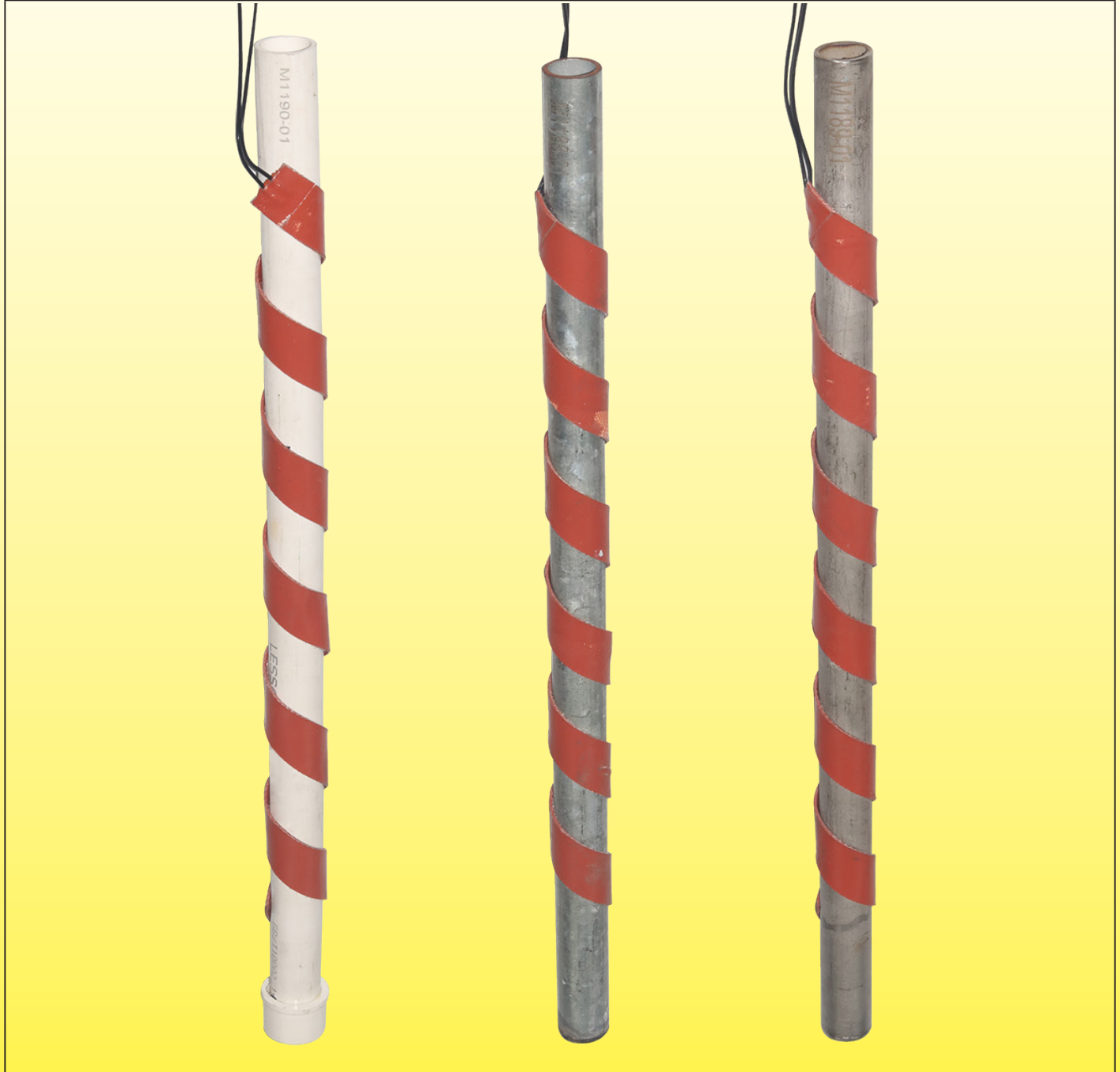
Condition of the comparative tests: Silicone heating ribbons wound on tubes of external diameter 25mm, in PVC-U, galvanized steel and stainless steel
