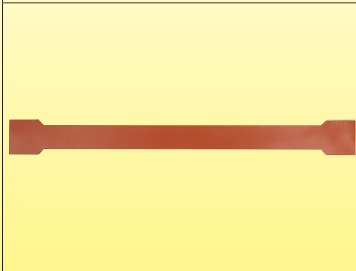
Type of sample tested (350 × 35mm)
